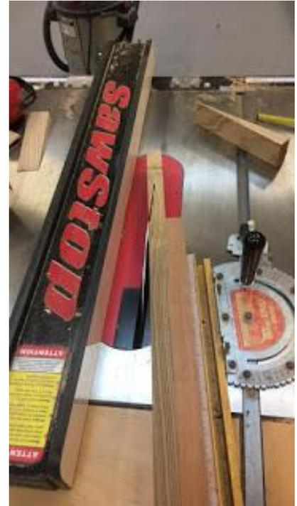
Yesterday I ripped catalpa wood for the balance of the parts for the Bevins Skiffs. I cut scarf joints on the table saw to extend sections of 8 foot stock to over 12 feet. I used epoxy glue thickened with wood flour to secure the joints. This stock, after being planed and cut to width and length will form the seat risers, and top rails. Today we can begin installing the frame pieces to which the seat risers and rails will be attached. The Inkra (brand) miter gauge shown is perhaps the only table
